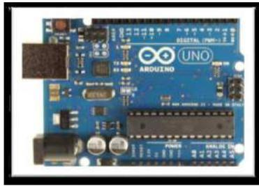
Gambar 3. Modul Arduino Uno
