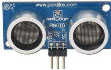
Gambar 2. Sensor Ultrasonik (PING)
