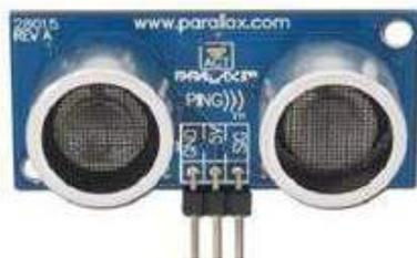
Gambar 2 Sensor Ultrasonik [2]
