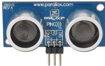
Gambar 2. Sensor Ultrasonik (PING)
