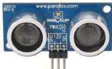
Gambar 2 Sensor Ultrasonik [2]
