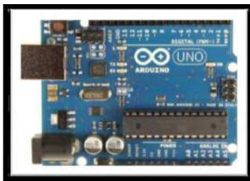
Gambar 3. Modul Arduino Uno
